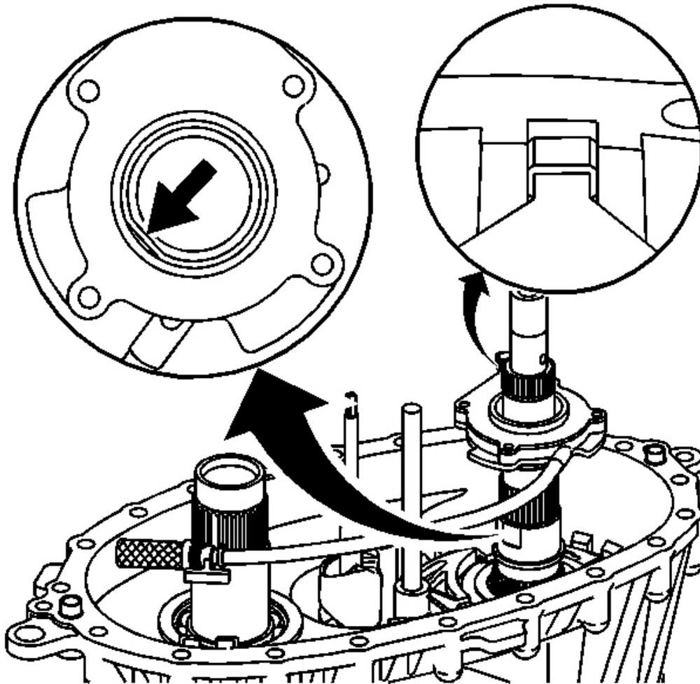
**Fig. 90: Expanded View Of Oil Pump Assembly**
