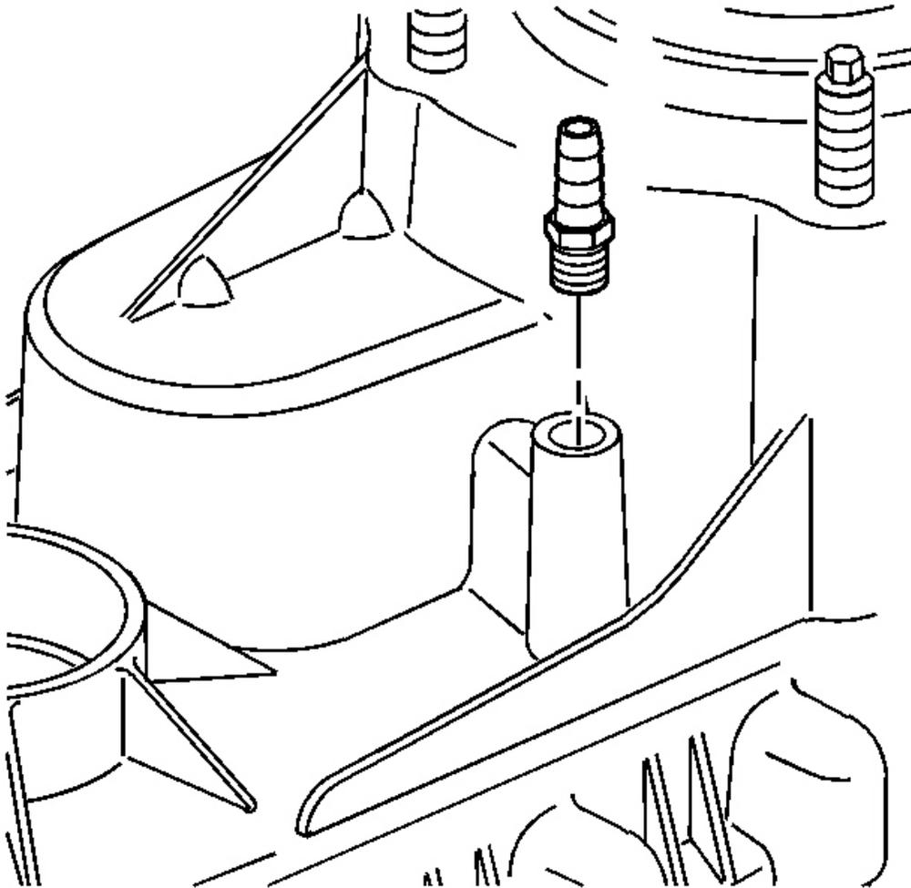
**Fig. 73: View Of Front Case Vent**
