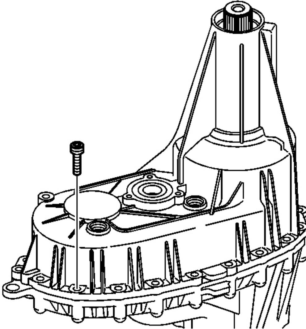
**Fig. 12: Identifying Transfer Case Retaining Bolts**
