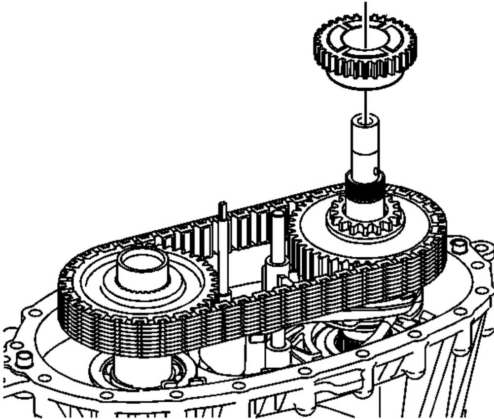
**Fig. 98: Identifying Front Sun Gear**
