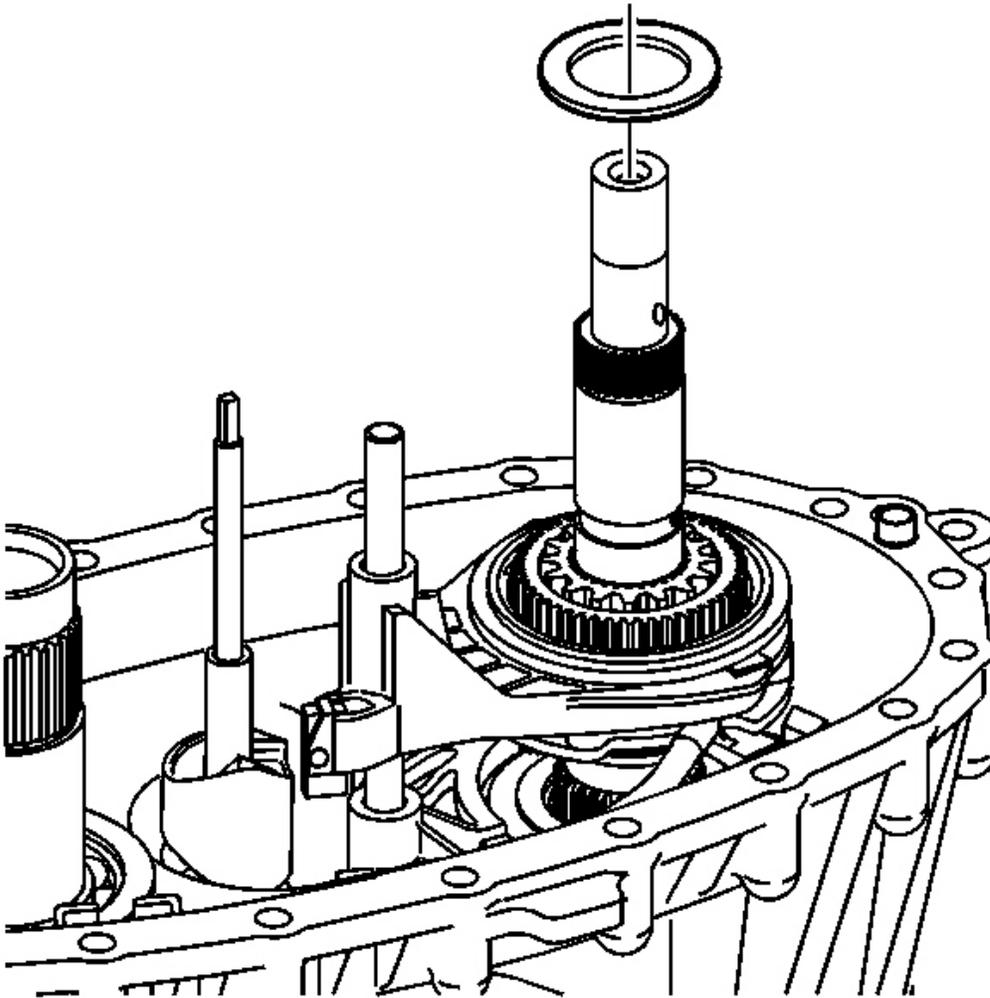
**Fig. 21: Identifying Drive Sprocket Thrust Washer**
