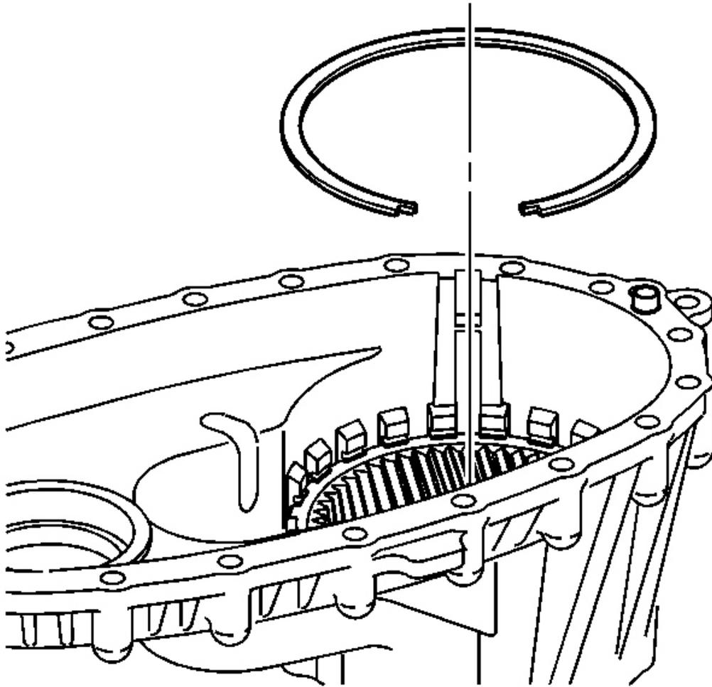
**Fig. 43: Locating Retaining Ring For Annulus Gear**
