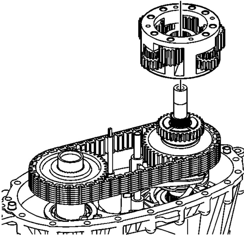
**Fig. 100: View Of Planetary Differential Assembly**
