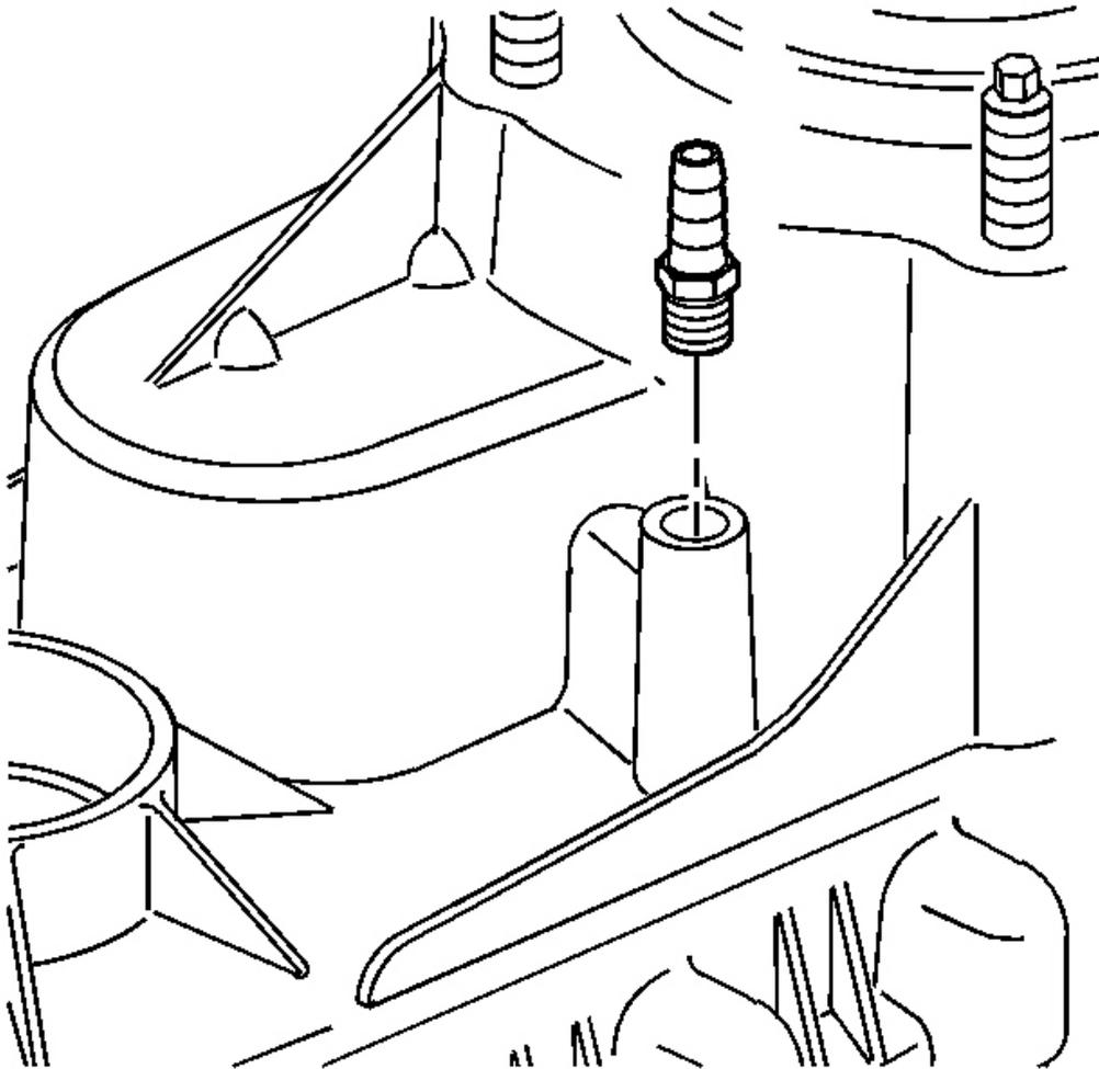
**Fig. 45: View Of Front Case Vent**
