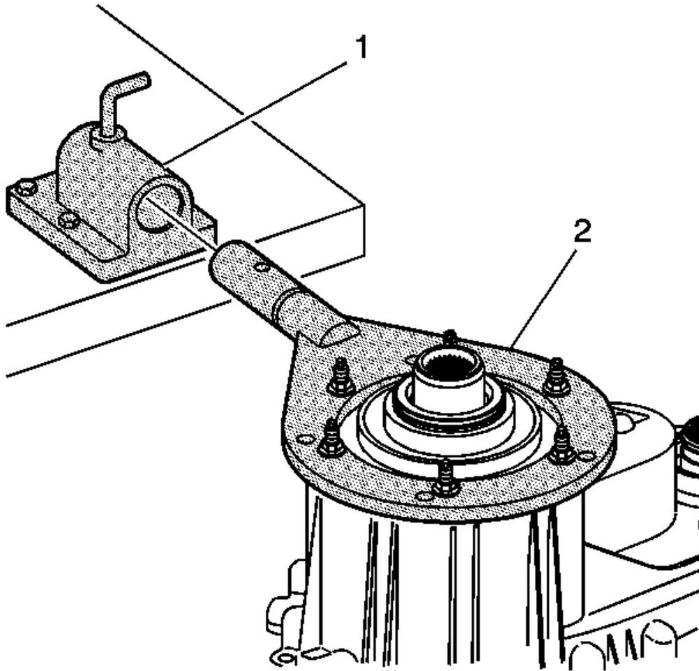
**Fig. 71: Installing J 45759 Into J 3289-20**
