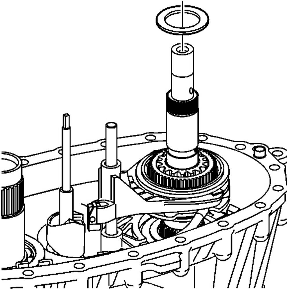
**Fig. 96: Identifying Drive Sprocket Thrust Washer**
