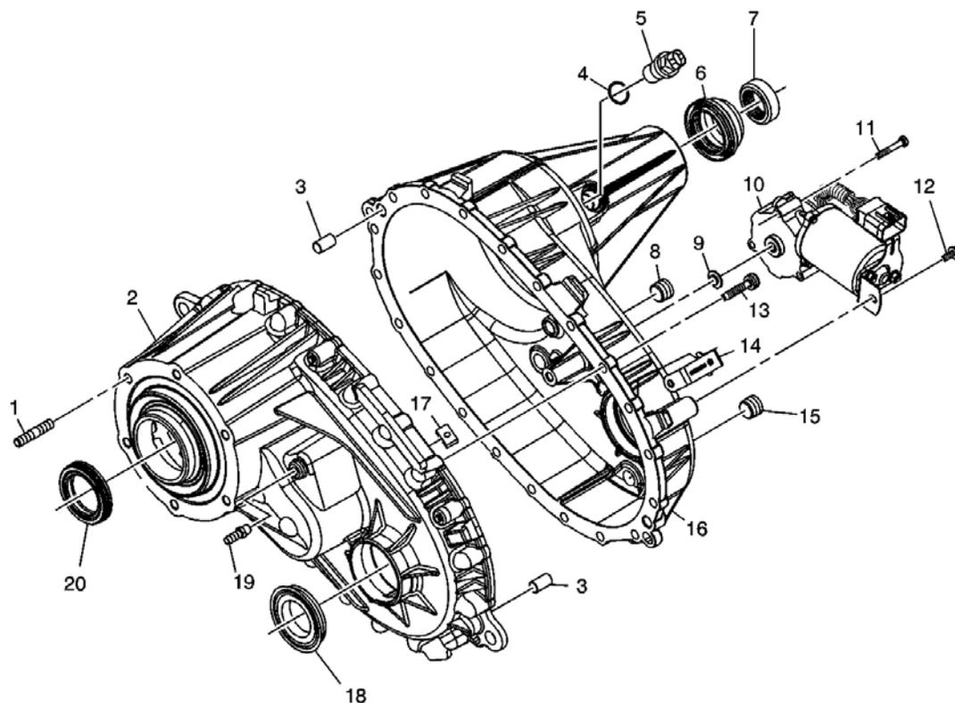
**Fig. 1: Case Components Disassembled View**
