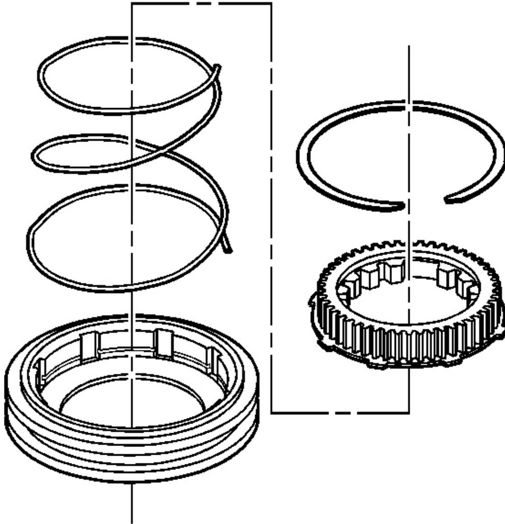
**Fig. 61: Illustrating Lockup Shift Assembly Components**
