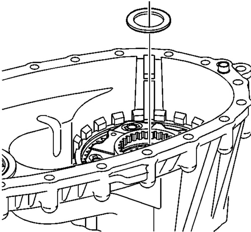
**Fig. 82: Locating Input Shaft Thrust Washer**
