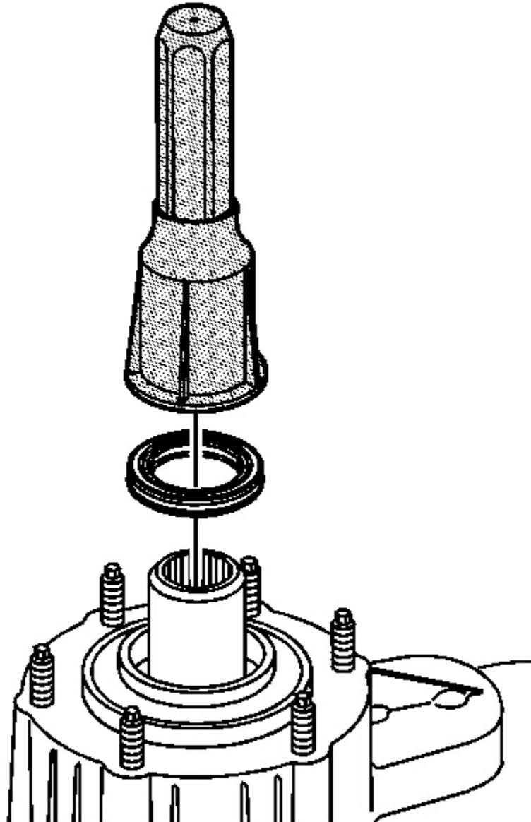
**Fig. 119: Installing The Front Input Shaft Seal J 42738**
