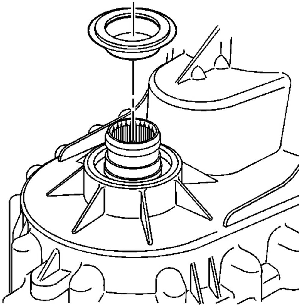
**Fig. 7: View Of Inner Seal Race From The Front Output Shaft**
