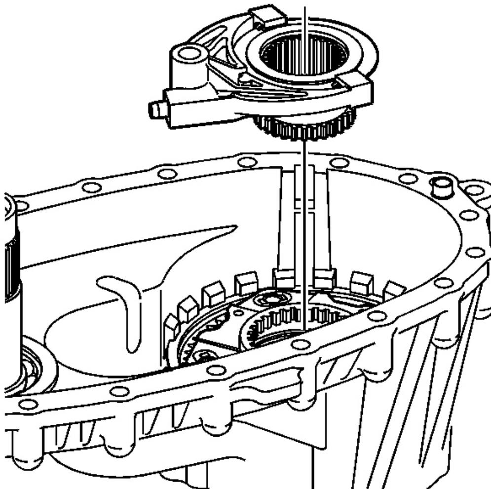
**Fig. 84: Identifying High/Low Range Sleeve With The High/Low Range Shift Fork**
