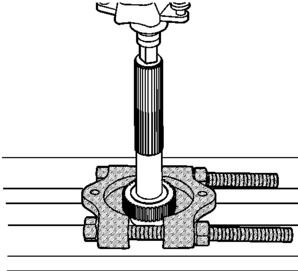
**Fig. 47: Removing Speed Reluctor Wheel With J 22912-01**
