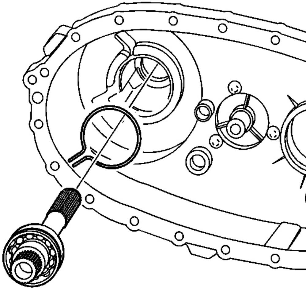
**Fig. 46: Identifying Rear Output Shaft & Outer Retaining Ring**
