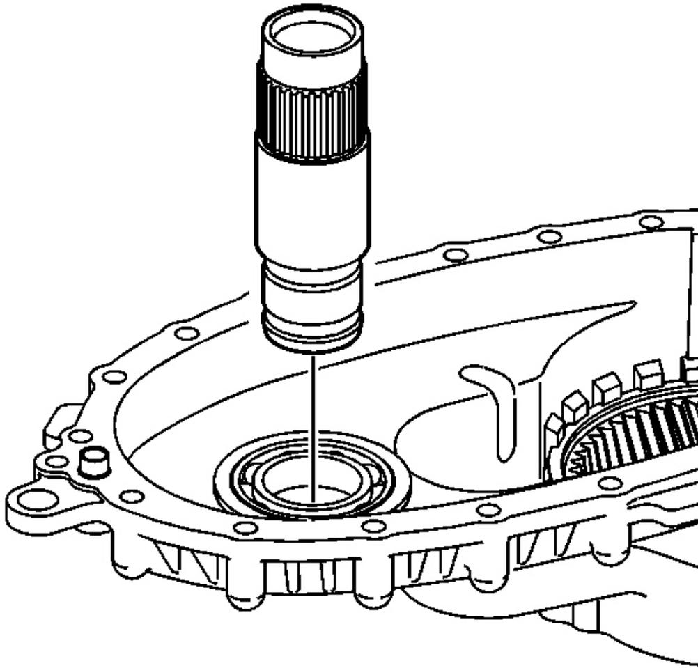
**Fig. 38: Front Output Shaft Assembly**
