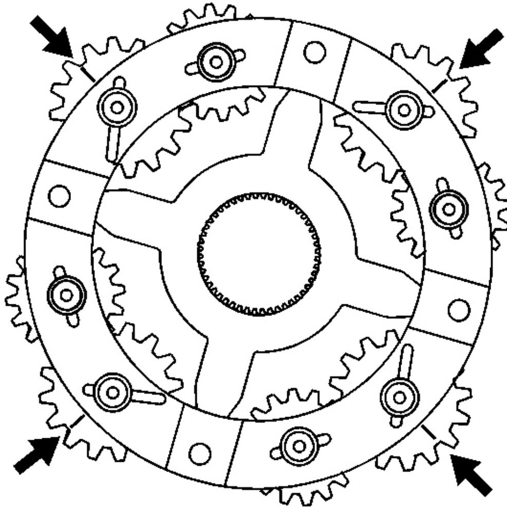
**Fig. 99: Aligning Marks On The Pinion Gears**
