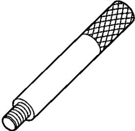
A universal driver handle with a threaded end, a smooth cylindrical middle section, and a knurled grip end. | J 8092<br>Universal Driver Handle                  |
