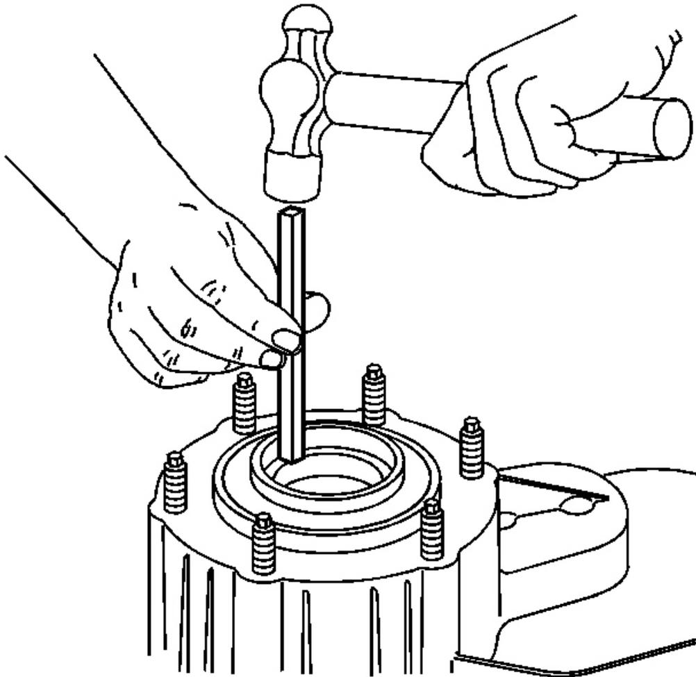
**Fig. 41: Tapping Out Input Shaft Bearing With Brass Drift**
