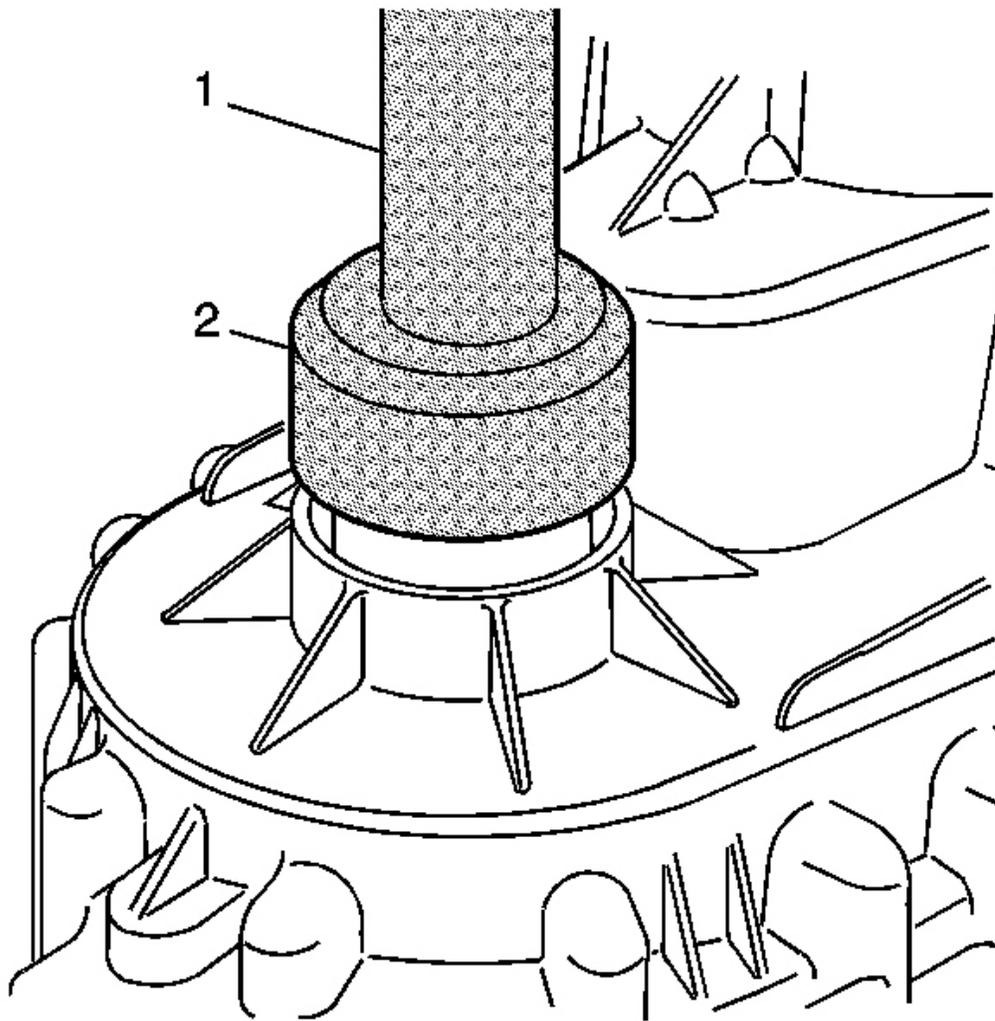
**Fig. 118: Installing Front Output Shaft Seal With J 43484 & J 8092**
