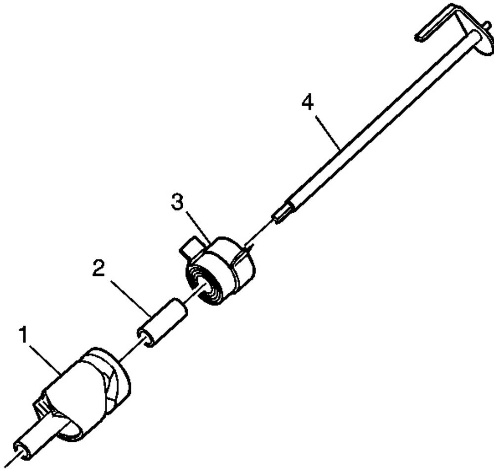
**Fig. 69: Expanded View Of Shift Detent Lever Assembly**
