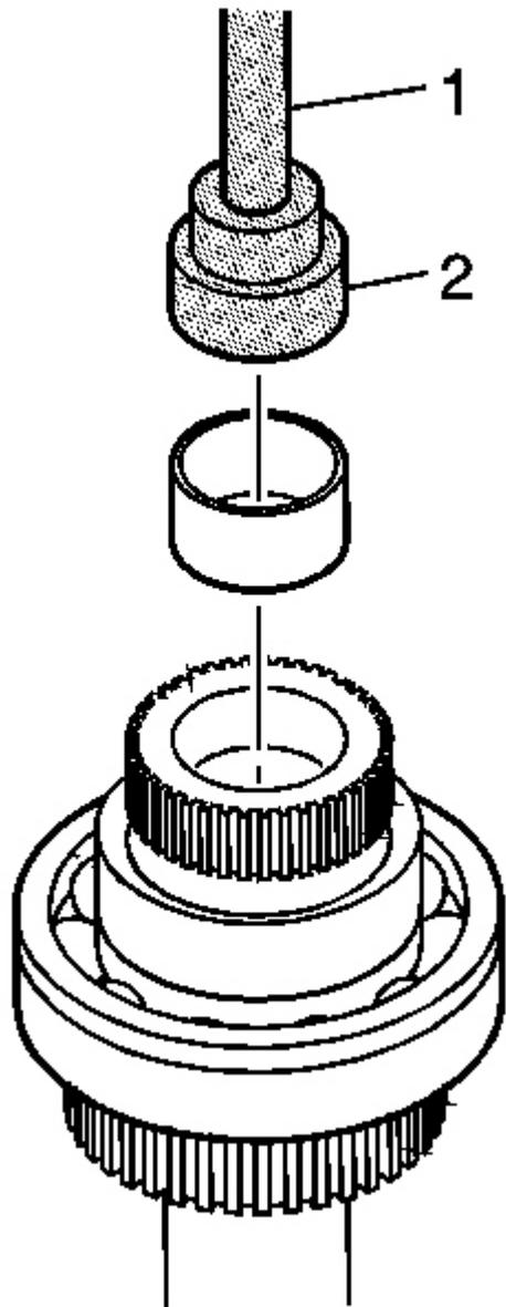
**Fig. 109: Installing Mainshaft Rear Support Bushing In Rear Output Shaft**
