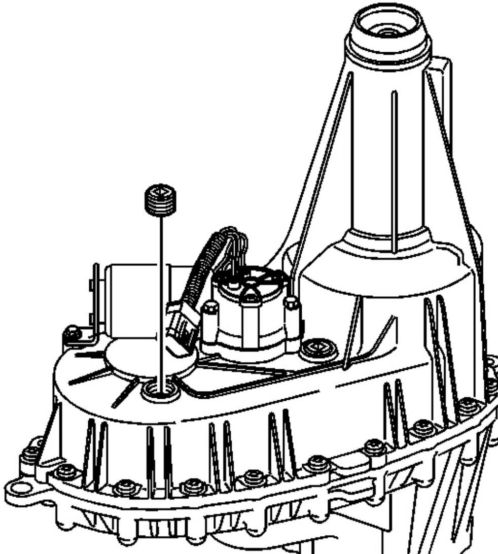
**Fig. 117: View Of Drain & Fill Plug**
