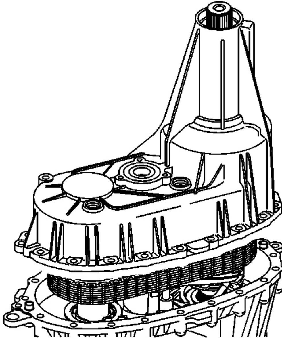
**Fig. 112: View Of Rear Case & Front Case Half**
