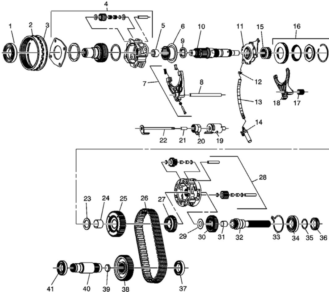
**Fig. 2: Transfer Case Internal Components Disassembled View**
