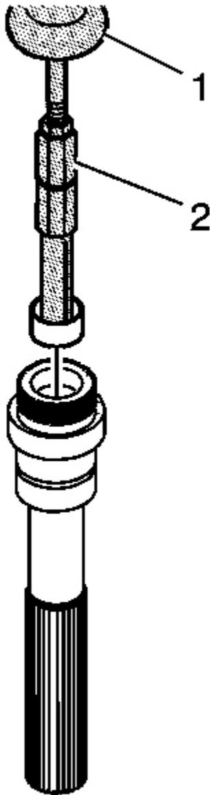
**Fig. 50: Using J 2619-01 & J 45548 To Remove Mainshaft Rear Support Bushing**
